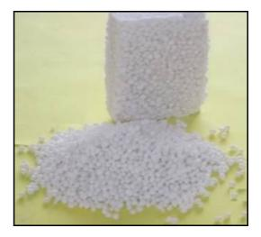
Block-shaped heat-insulated material is produced on the base of grain foamed granules and binder. The material can be applied as an efficient heat-insulated material for dwelling and industrial constructions, industrial equipment and pipelines, large capacity transport.
